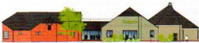
View of 2011 proposals for new Budgens store from the Winchester Road. Showing timber cladding over brickwork to east and new windows to frontage
